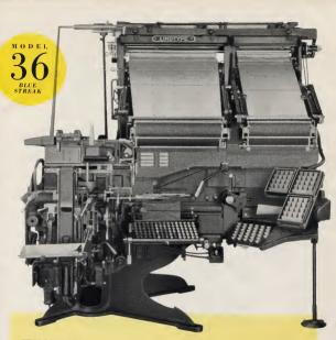
THE EQUIVALENT of the Mixer Model 35 Super Display, plus auxiliary magazines. Its Wide-Standard magazines (35% wider Hum standard magazines) and wide 34-channel auxiliaries facilitate the keyboarding of either straight matter, mixed or display composition with equal ease.
